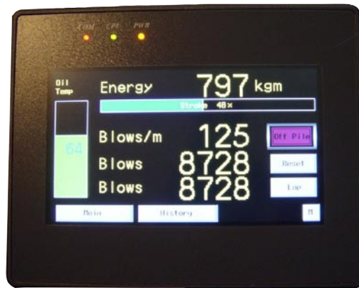
INTERFACE SCREEN MOUNTED ON POWER PACK
